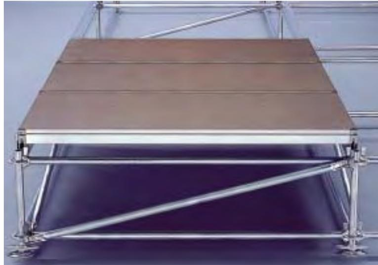
Starting from a basic unit, each podium grows by the system dimensions (2.07 m x 2.57 m; 2.07 m x 2.07 m or metric) to the required size. Side guard rails are installed, made either from Allround system scaffolding parts the same as the substructure or from standard-production guard rail parts, also with child protection feature.
