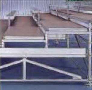
The Event transom support ensures that the 2.57 m bay has a 7.5 kN/m<sup>2</sup> load-bearing capacity; the Event stand element determines the rise and supports the Event decks.
